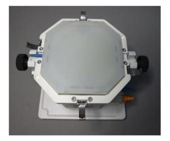
Close the cover, the position pin's of the cover fit in the unit top
