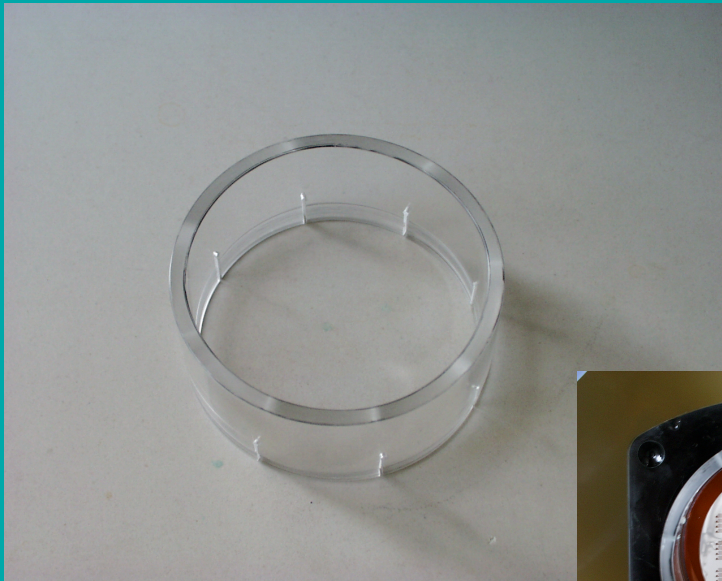
Shield (for more homogeneous layer growth)
